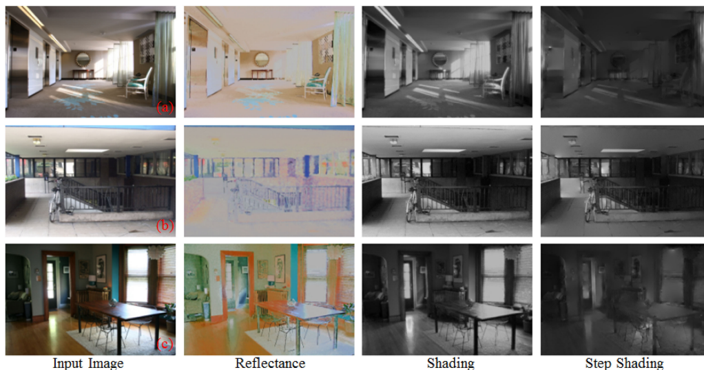
Fig. 16. Visual results of intrinsic images recovery on real scenes. We chose three scenes (a), (b), and (c) from a real-world dataset IIW [17]. (a) shows that our method deals with an indoor scene with complex illumination. (b) is an outdoor scene. As shown in (c), in the bright region of the table, there is residual in the reflectance. Overall, our method achieves promising results on real-world images.
