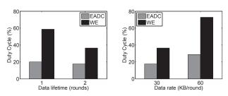
(a) Duty cycle as a function of (b) Duty cycle as a function of data lifetime amount of data
