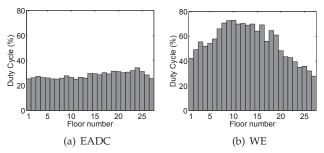
Fig. 20. Duty cycle of each sensor in the building with 27 floors.
