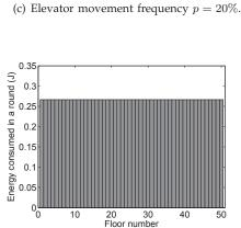
(c) Elevator movement frequency p = 20%.
