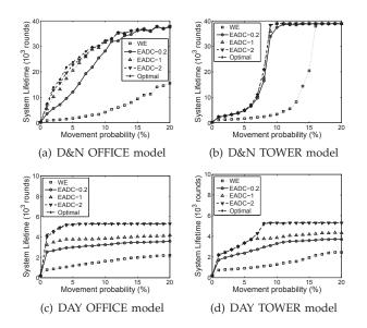
Fig. 10. System lifetime as a function of the elevator movement probability, i.e., p in the building with 20 floors.
