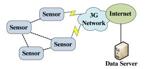
Fig. 1. The architecture of the wireless sensor network using 3G transmission.
