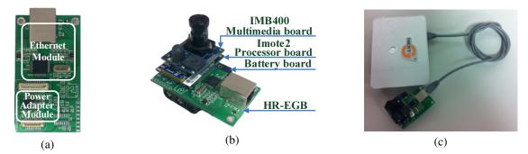
Fig. 2. Our Long-range High-rate communication module for Imote2
