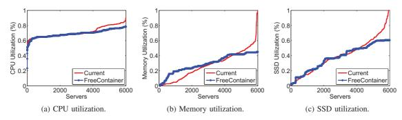
Fig. 5: Resource utilizations of the Baidu server cluster before and after deploying FreeContainer.
