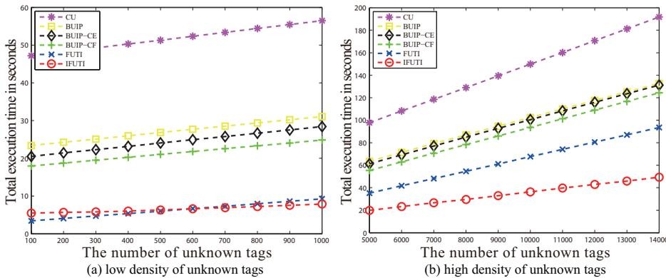
Fig. 4: Evaluating the execution time of the proposed protocols, where the number  $N$  of known tags is fixed to 10,000; and the identification accuracy  $\alpha$  is predefined as 99%.
